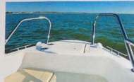
BOW: The split pulpit permits boarding over the bow using the proper boarding step over the chain locker.
