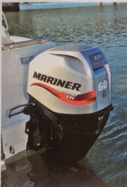
POWER: Mariner 60hp is the maximum rated for the boat.
