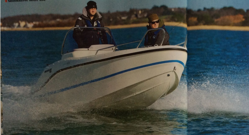
CONSOLE: The wheel is placed close to the centre line to keep the lateral weight distribution even.
