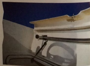
SEAT: The seat lid is supported by a gas strut and houses the lighting mast.
